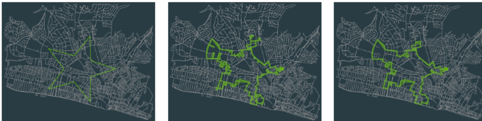
Figure 7: An example of the results from the snapping algorithm and dead-end removal
